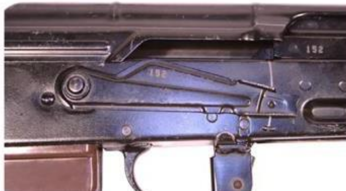
Figure 8. The Selector Lever Placed on AUTO.
