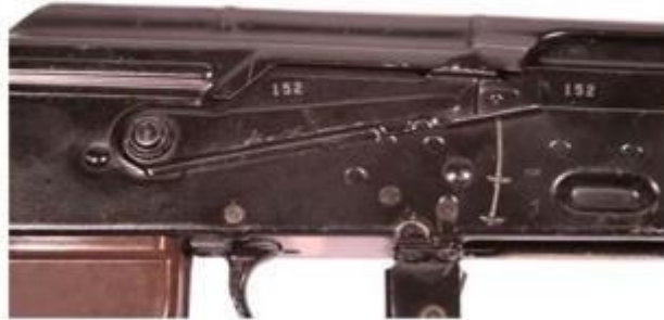
Figure 6. Selector Lever Placed on SAFE.
