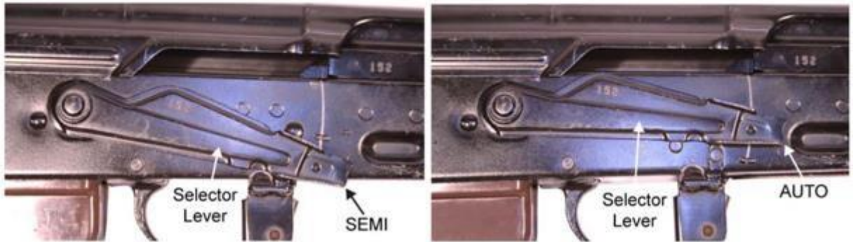
Figure 3. Selector Lever on SEMI (left) or AUTO (right).
