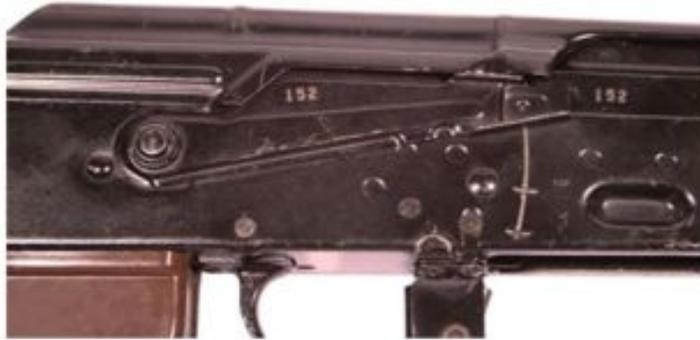
Figure 6. Selector Lever Placed on SAFE.
