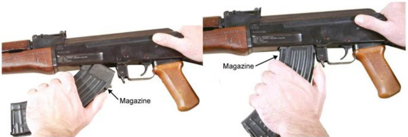
Figure 1. Inserting a Magazine.
