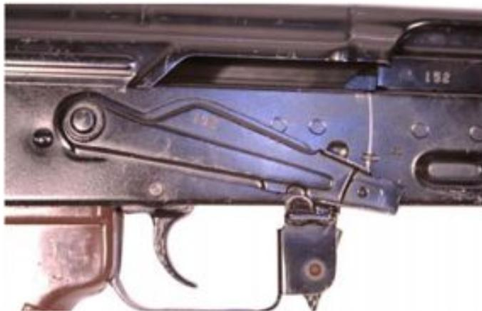
AUTO. When the selector lever is placed on AUTO, the weapon will continue to fire as long as the trigger is held to the rear or until the magazine is empty. The selector lever must be set on SEMI or AUTO to chamber a round or to clear the weapon. Refer to in Figure 8.
