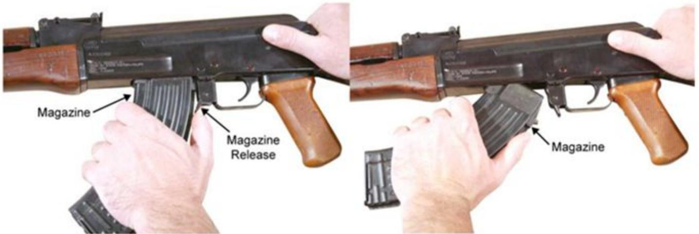
Figure 2. Removing the Magazine.
