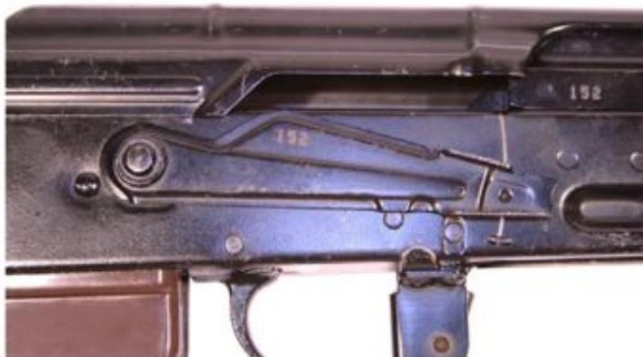
Figure 8. The Selector Lever Placed on AUTO.
